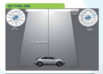
When an object is in the detection area, the sensor tube turns on
