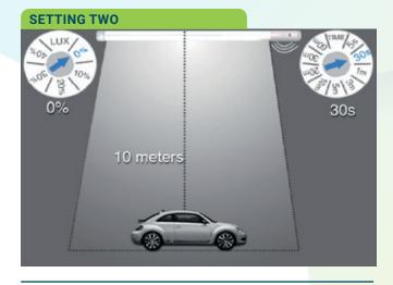
When an object is in the detection area, the sensor tube turns on
