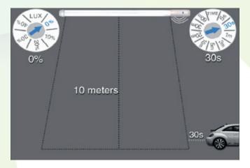
When an object is away from the detection area, after 5 minutes the sensor tube reduces to 20% and consumes 3.5 watts.
