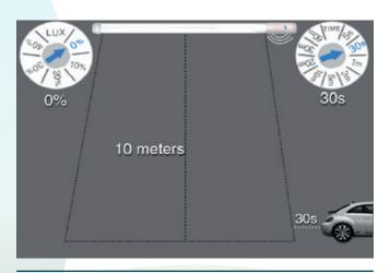
When an object is away from the detection area, the sensor tube turns off after 30 seconds.
