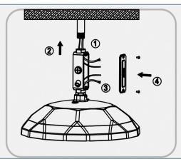
Thread the wire into the junction box, install the junction box on the pipe, wire according to the requirements, take protective measures, and lock the cover.
