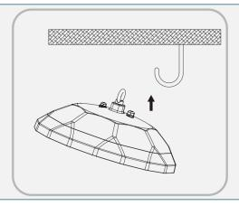
2. Put the ring into the mounting hook.
