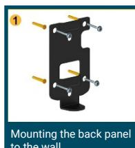
Mounting the back panel to the wall
