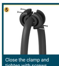
Close the clamp and tighten with screws
